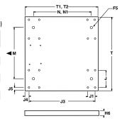
1NA Mounting Table Top (2) (Custom mounting hole. Dimensions in mm)
