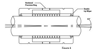
Super Smart Ball Bushing Bearing Self-Alignment Feature
