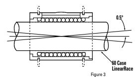
Super Ball Bushing Bearing Self-Alignment Feature
