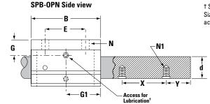
† Size .500 has oil lubricant fitting. Sizes .625 and above have 1/4-28 access for lubrication.
