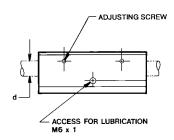
Super Smart Twin Pillow Blocks (Open Adjustable Type) (Dimensions in mm)
