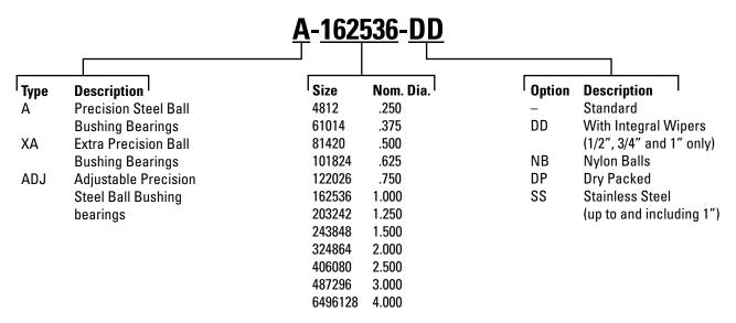
Precision Steel Ball Bushing Pillow Blocks (Closed Type) for End Supported Applications
