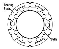
Cross-section of Super Ball Bushing Bearing
