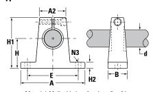
Material: Malleable Iron for sizes .5 to 2 in. Aluminum Alloy for sizes .25 and .375 in.
