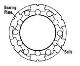
Cross-section of Super Ball Bushing Bearing
