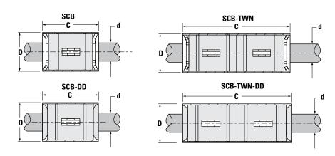
Super Ba Bushing Cartridge Bearings and 60 Case LinearRace (Dimensions in inches)
